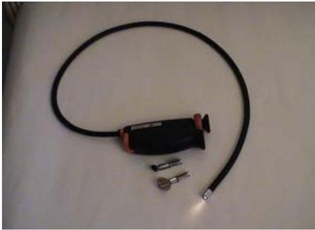
By super gluing a larger mirror to the Testo mirror you can improve the quality of the view.
