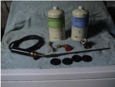
**Sensit H.E.T. Kit came with regulator, hose, distribution wand, hole plugs, tracer gas and calibration gas for the HXG-2**
