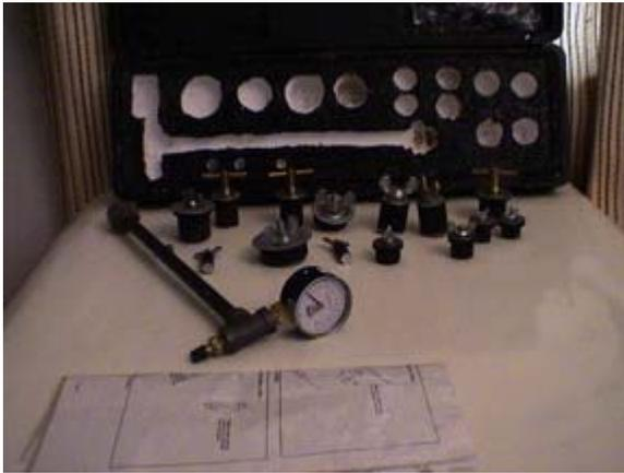
The kit comes with the pressure gauge fixture, plugs, instructions and a furnace wall patch plate. Additional patch plates available in a package of 5 using part number 16L98 can be ordered through Lennox. The plugs can also be used to block off standing tees on air conditioning drains so you can use a sludge sucker at the drain end to clear plugs.
