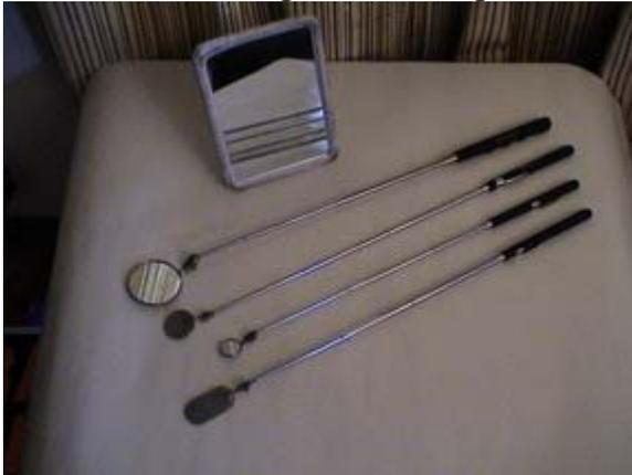
For older heat exchangers have a mirror made at local glass shop 1/4" thick x 1-3/16" width x 24" length. A suitable carrying case can be made from 1-1/4" PVC pipe and fittings. Use a male threaded cap for one end. Install a small piece of foam such as rubatex in both ends. A tool plastic coating can be sprayed on the back side for protection and at one end for a hand grip.
