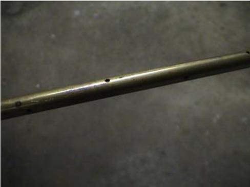
**The wand is a brass tube closed off at one end with several dispensing holes drilled into it.**
