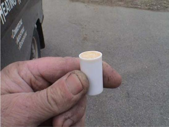
Using a smoke puffer you can fill the burner chamber with smoke. Then turn the blower on. If the smoke sprays out and away from the burner opening you have a good indication of a leak in the heat exchanger.
