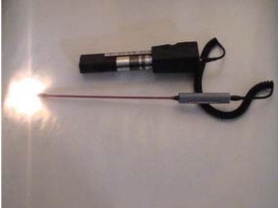
Shining a light on the outside or the inside of the heat exchanger at the suspected area and examining the opposite side look for light penetration through the crack or perforation.
