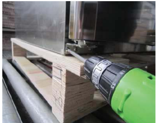
H. Assemble the door, then rotate it about 180 degrees. Assemble top hinge(right) with stopper plate in bottom hinge (left) position. (First, assemble top hinge (left); second, assemble bottom hinge (left) while doors are closed, insert hinge into door bushing(left) with lifting, rotate doors counter-clockwise, screw hinge in original positions.)
