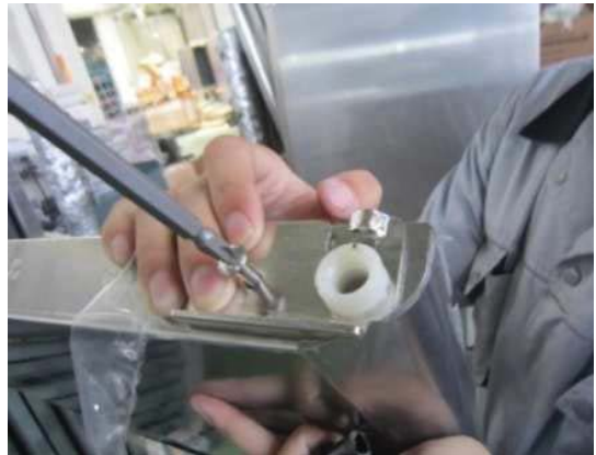
H. Assemble the door, then rotate it about 180 degrees. Assemble top hinge(right) with stopper plate in bottom hinge (left) position. (First, assemble top hinge (left); second, assemble bottom hinge (left) while doors are closed, insert hinge into door bushing(left) with lifting, rotate doors counter-clockwise, screw hinge in original positions.)
